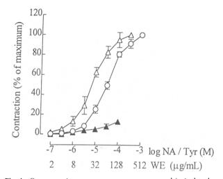
**Fig. 4.** Concentration-response curves constructed in isolated vas deferens preparations to noradrenaline (NA,  $\circ$ ), the water extract of *Piper marginatum* Jacq (WE,  $\triangle$ ) and tyramine (Tyr,  $\blacktriangle$ ) after the extract. Symbols and vertical bars are means  $\pm$  s.e.m. of 5 experiments in each group.
